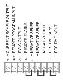
FOR LOCAL VOLTAGE SENSING, CONNECT (S+) TO (E+) AND CONNECT (S-) TO (E-) FACTORY INSTALLED JUMPERS ARE PROVIDED.
