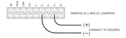
FOR IMPROVED VOLTAGE READBACK, USE THE REMOTE VOLTAGE SENSING CAPABILITIES.
